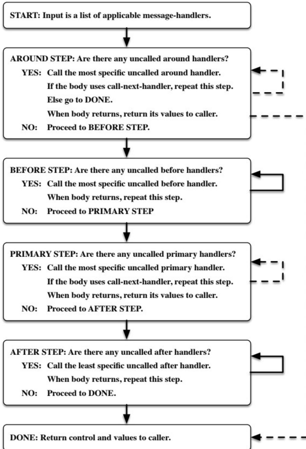
The solid arrows indicate automatic control transfer by the message dispatch system. The dashed arrows indicate control transfer that can only be accomplished by the use or lack of the use of **call-next-handler** (or **override-next-handler**).
