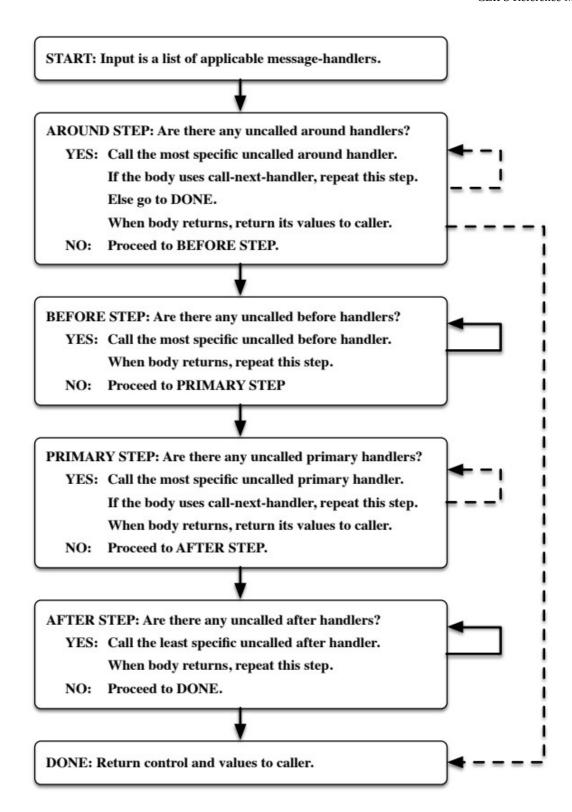
The solid arrows indicate automatic control transfer by the message dispatch system. The dashed arrows indicate control transfer that can only be accomplished by the use or lack of the use of **call-next-handler** (or **override-next-handler**).
