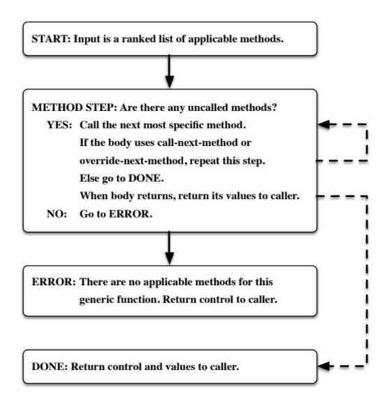
The solid arrows indicate automatic control transfer by the generic dispatch. The dashed arrows indicate control transfer that can only be accomplished by the use or lack of the use of call-next-method or override-next-method.
